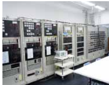
Power system simulator at Waseda University in Tokyo, which is used for the practical training class in the "Basics of Power Supply Network Systems"
