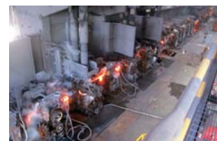
A steel bar manufacturing line (ISPC of the Al Tuwairqi Group)
