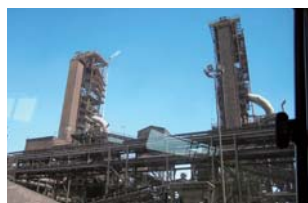
A direct reduction iron (DRI) making plant (DRIC of the Al Tuwairqi Group)
