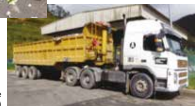
Waste carrier vehicle (Loading capacity: 20 tons)
